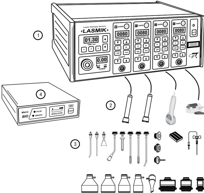
Fig. 5. Modular design concept of low-level laser therapy equipment
